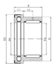
NKX 25 Z Bearing 2D drawings and 3D CAD models
